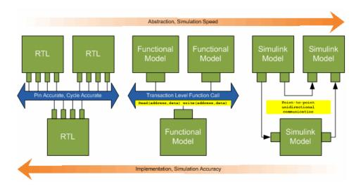
The functional model provides a sort of halfway point between the speed you can achieve with abstraction and the accuracy you get with implementation.
